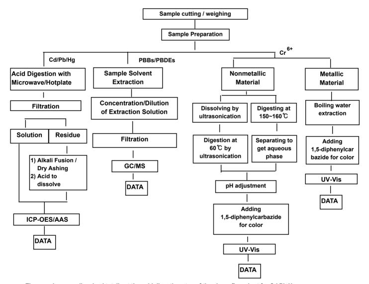
The samples were dissolved totally at the acid digestion step of the above flow chart for Cd,Pb,Hg
